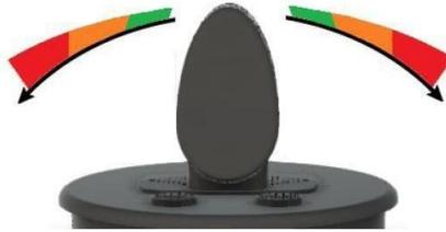
4. *Note: It is only possible to thrust to Port or Starboard side when the thruster is detected to be fully deployed.*
